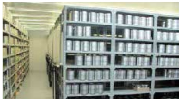
The new 21 degree celsius storage room where some of the canned horse mackerel was kept during the three-year testing period
