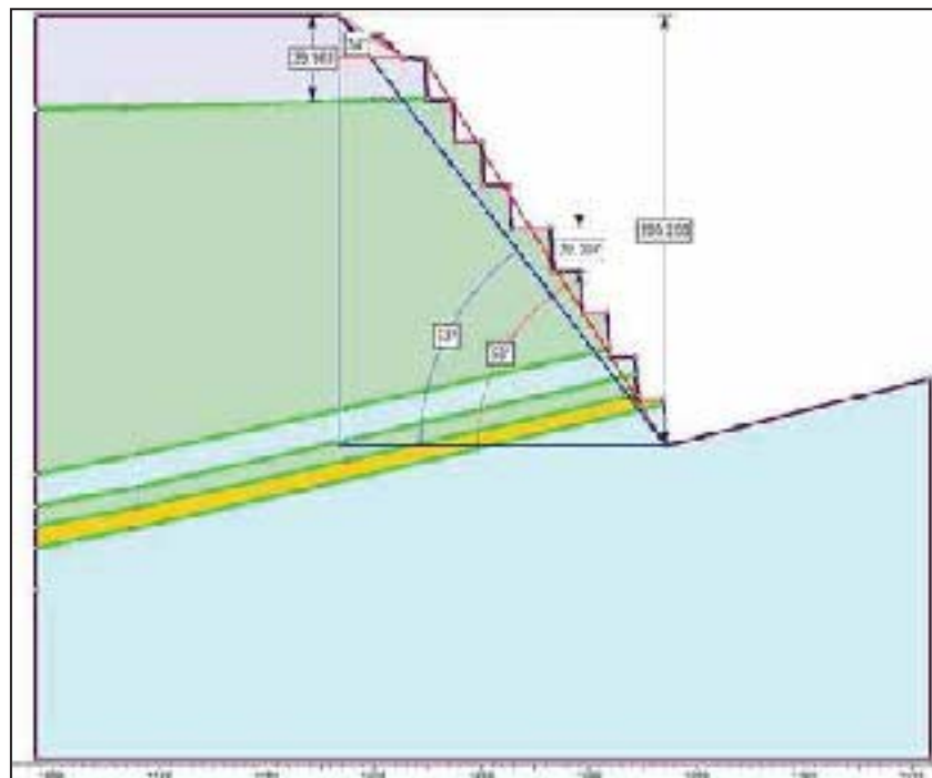
Figure 9.2.2_8 The Proposed Final Pit Slope Design
