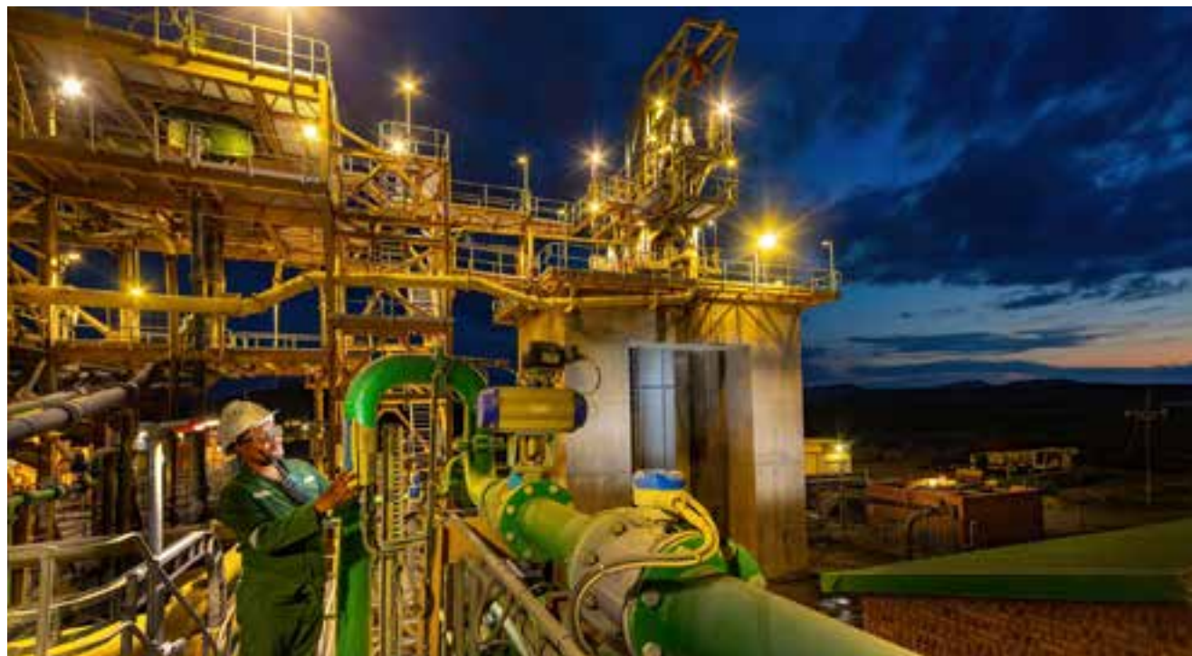
The HIGmill, a high intensity grinding mill, at the Maseve concentrator
