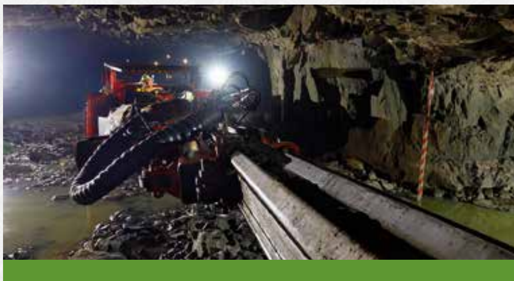
A drill rig, which is part of Styldrift's trackless fleet, drilling on 600 Level
