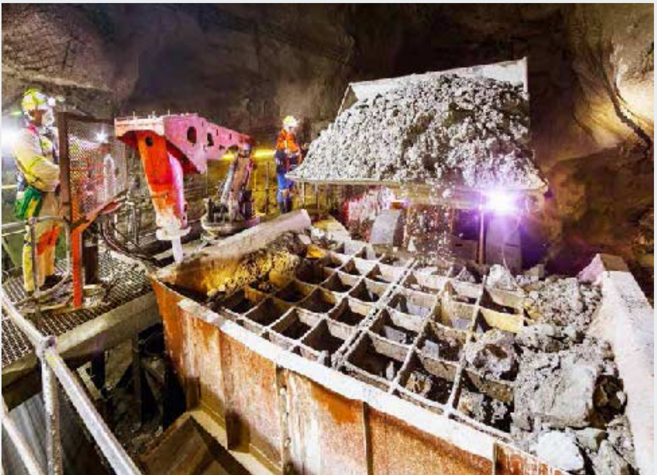
Tipping of ore in Phase III 114 level hybrid mining section at BRPM
