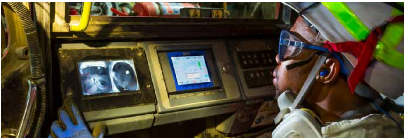
Cameras used together with collision avoidance technology
