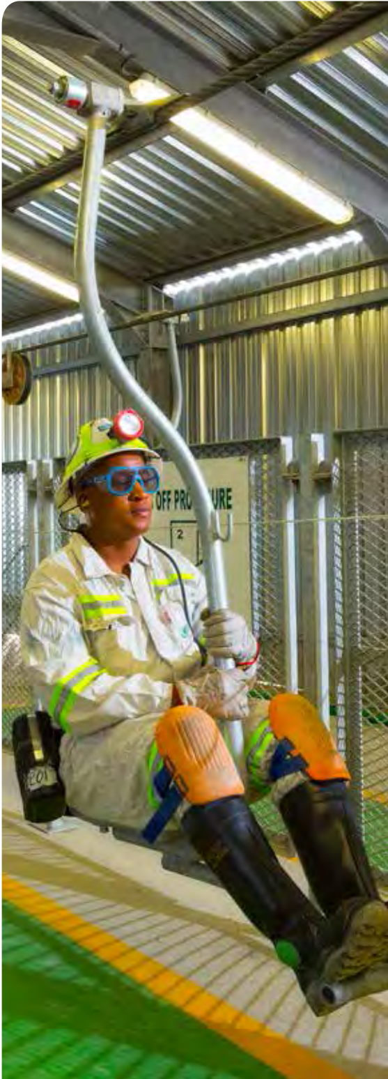
The chairlift at BRPM's North shaft was installed to provide employees with safer and faster transportation into the mine.
