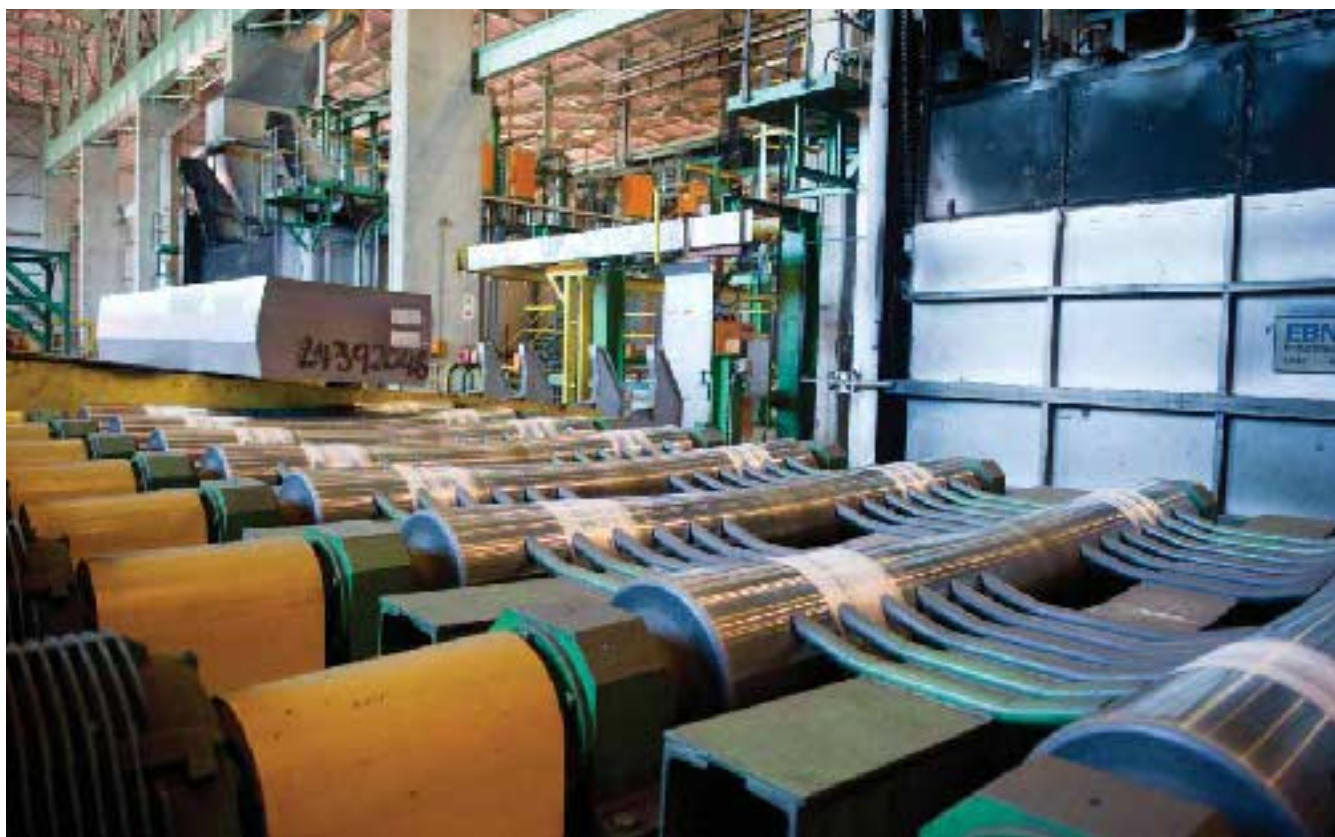
Aluminium rolling slab loaded onto Hot Rolling bed after scalping and preheating (refer page 4)
