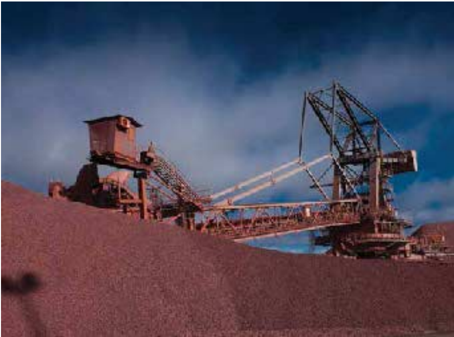
01 The stacker-reclaimer at Kolomela mine assists in the blending of different grades of processed ore prior to shipment.
