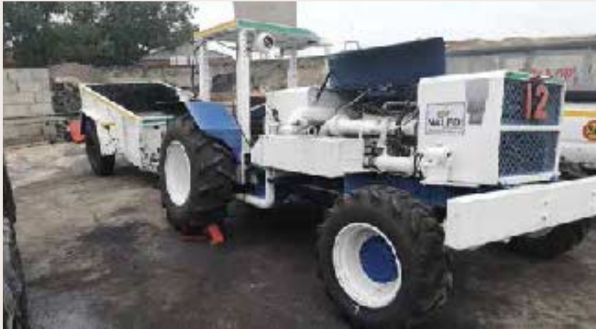
Tractor-trailer for transporting building material underground
