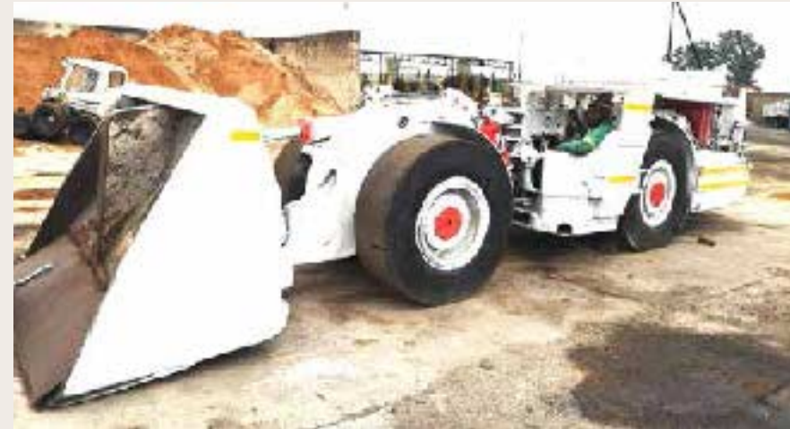
Load-haul dumper transports building material underground, doubles up for cleaning the area before work starts
