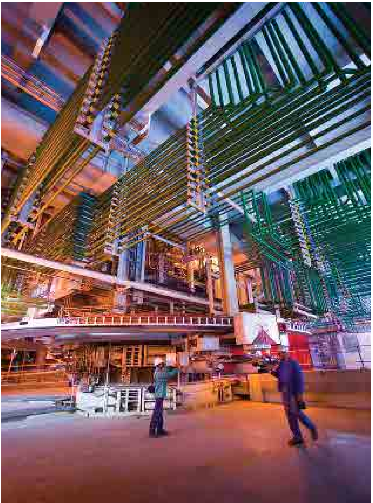
Metallurgist Neo Molelekeng inspecting the thermocouple connections and mud-guns at the ACP Phase B furnace.
