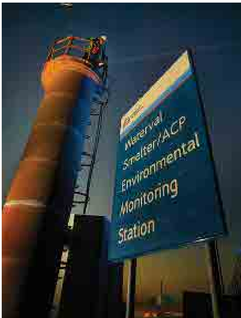
Donovan Rieger inspects the Waterval Smelter fence-line \text{SO}_2 monitoring equipment. This technology uses light diffraction to determine ground-level \text{SO}_2 emissions.
