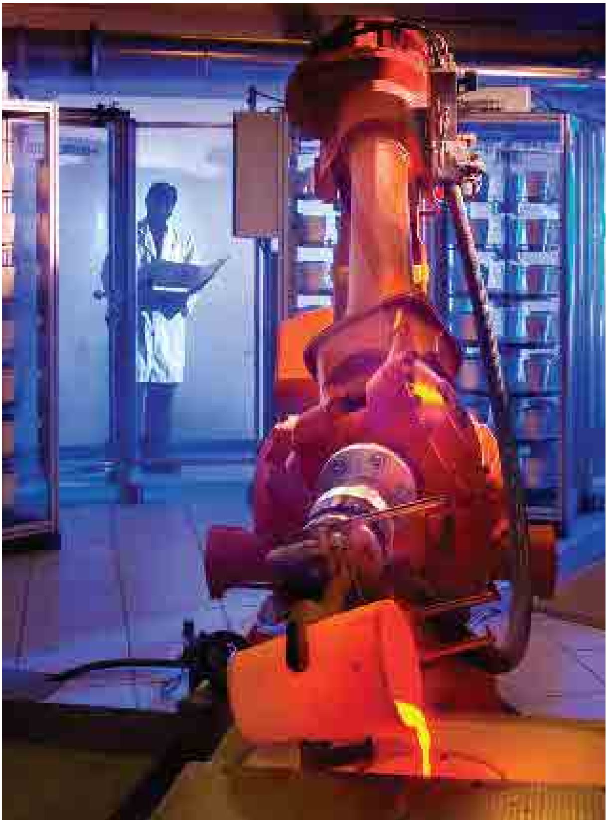
Comfort Kupa, an instrument technician at PPRust, monitoring crucibles in the robolab.
