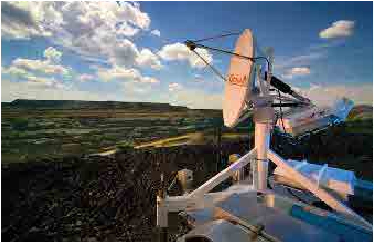
A sophisticated radar and laser system in use at PPRust's open pit to monitor slope stability. Radar and laser beams detect the slightest movements in rock stability. The system is able to alert pit management of any potential rock fall, thereby enhancing pit safety.
