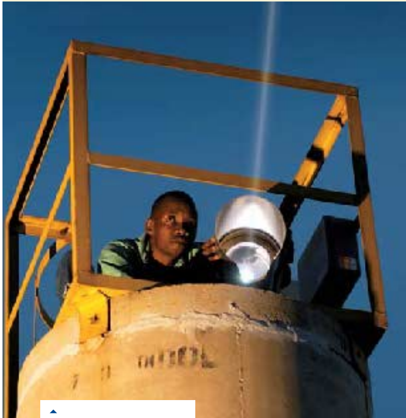
Occupational Hygiene Assistant Abraham Makodi adjusting the alignment of the Fenceline Monitoring System's laser light to target a distant receiver at the perimeter of the ACP and Waterval Smelter complexes. The system monitors gases and airborne particles which pass through the beam.
