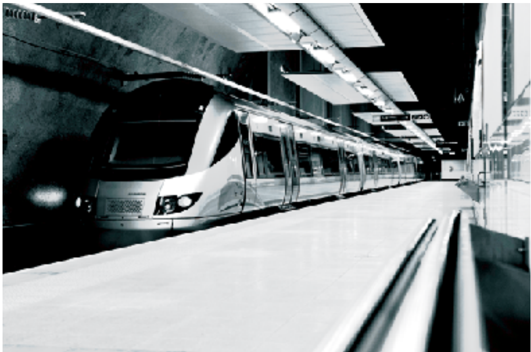
The Gautrain – Stainless steel has been used throughout the station for its ability to withstand wear and tear. It is also easy to clean. The seat in the foreground is made of stainless steel.
