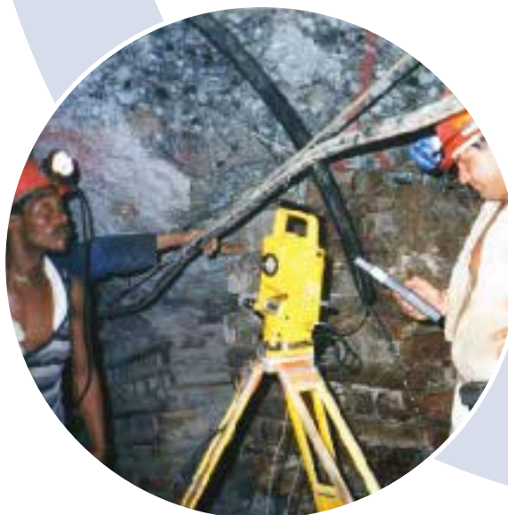
Rutherford – measuring angles and distance underground
