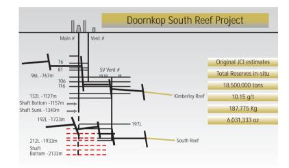
The ventilation shaft, which will also be used as a second outlet, has been completed. The main shaft has only been sunk to a depth of 1336 metres with the final depth 2 135 metres below surface.
