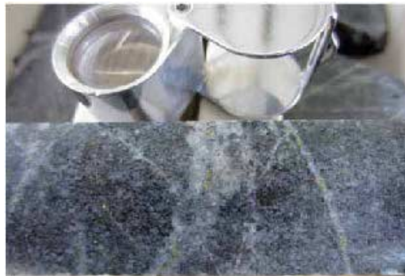
Figure 2: PNDD001; 599m. Biotite altered metasediments with quartz vein stockwork containing chalcopyrite, molybdenum, pyrite and magnetite. Assays pending.
