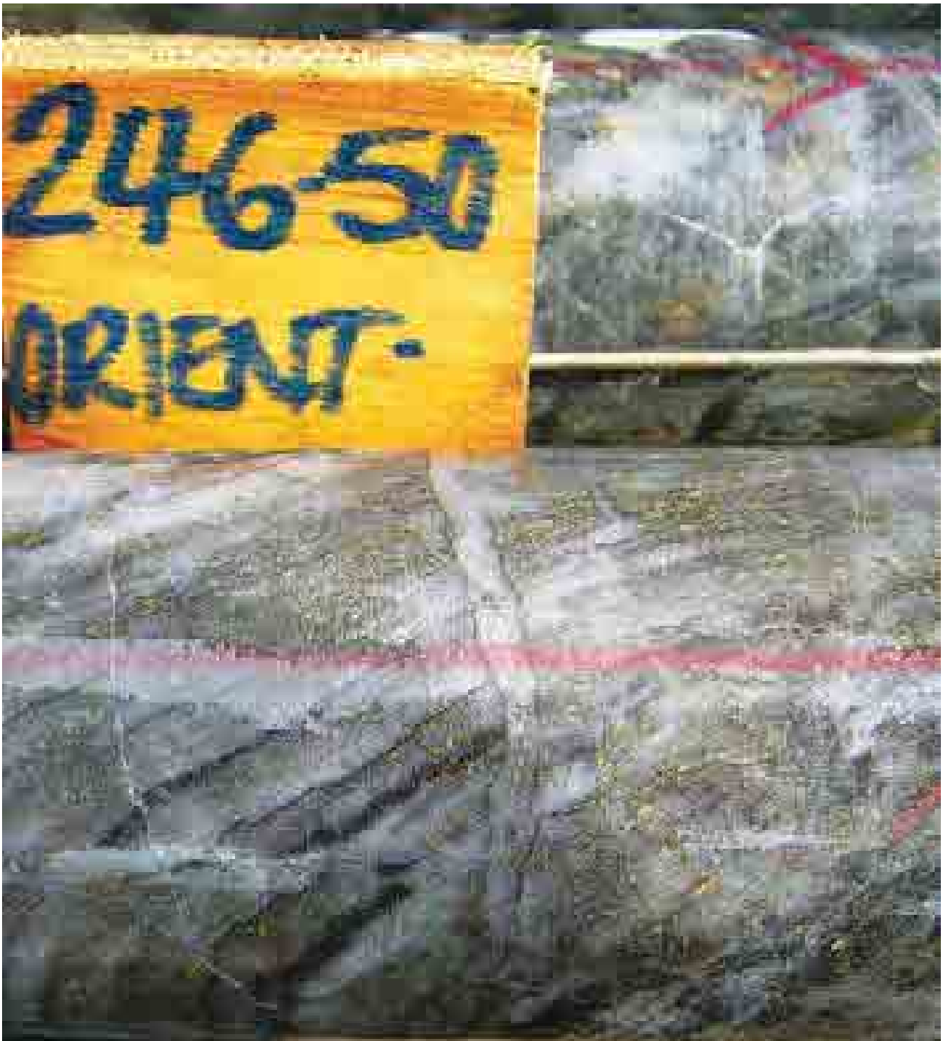
WR262; 246.5m. Banded quartz magnetite chalcopyrite vein stockwork developed in metasedimentary rocks of the Owen Stanley Metamorphics. Assays for this interval (246 – 247m) returned 2.9 g/t gold and 0.7 % copper.
