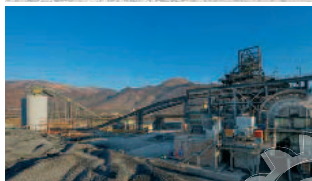
Two Rivers primary mill and primary mill feed system
