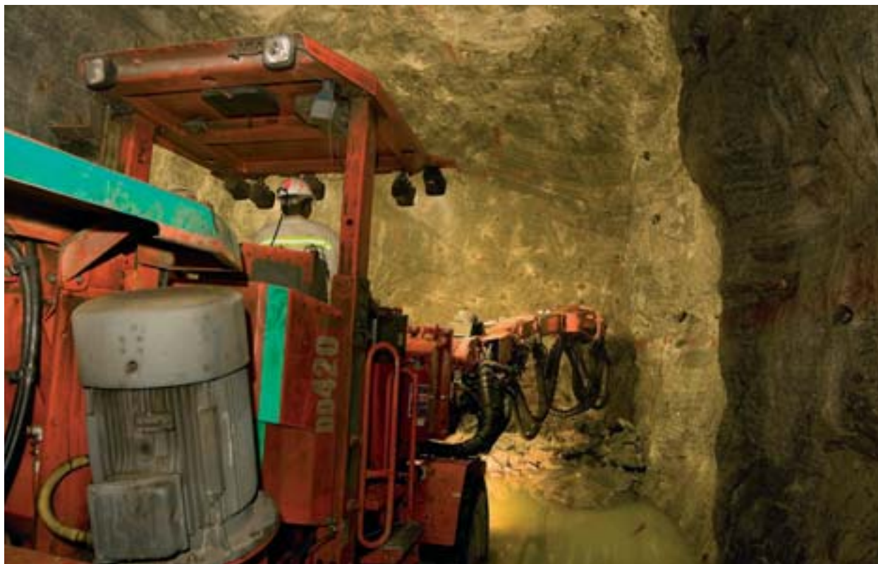
Modikwa Platinum Mine development end drilling
