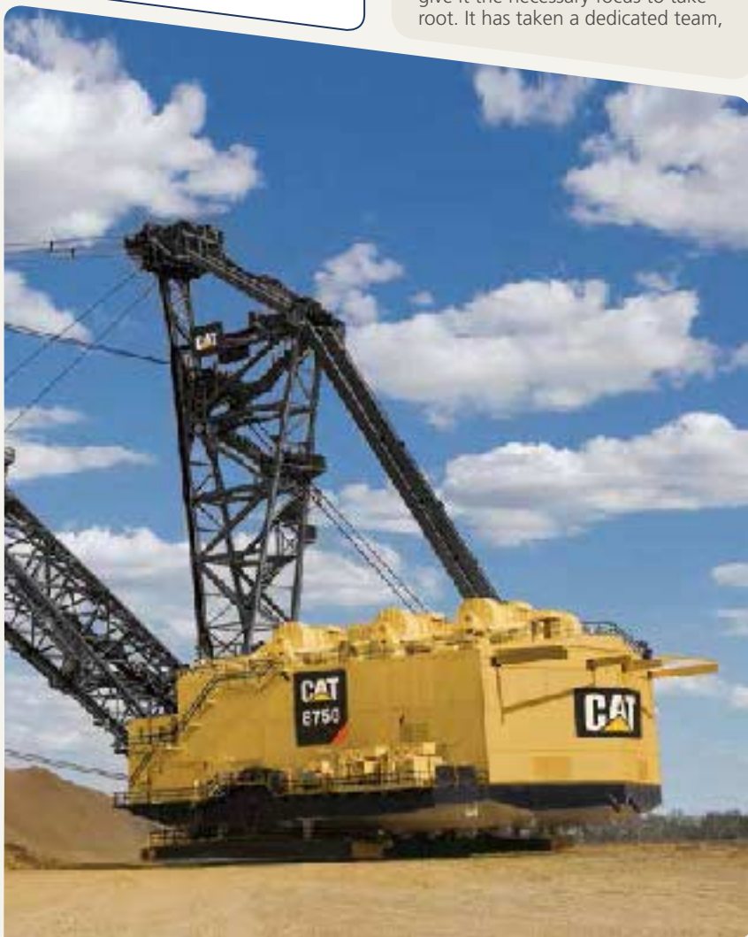
A Cat dragline, an important excavating tool used in many surface mining operations worldwide. One of the new machines offered in the EMPR range, the Cat dragline offers the lowest material removal cost per tonne and an average operating life of 40 years.
