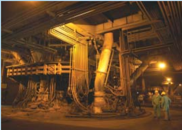
Furnace no. 2 which was completely rebuilt after more than 30 years service
