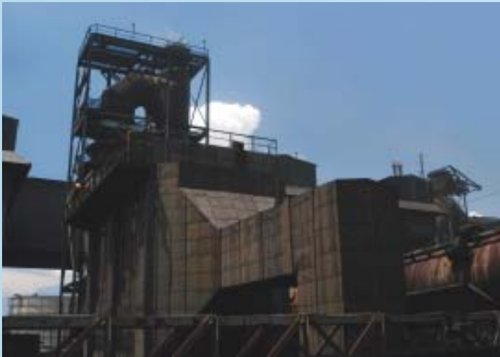
A refurbished kiln off-gas precipitator which is one stage of the current emissions reduction programme for the iron plants
