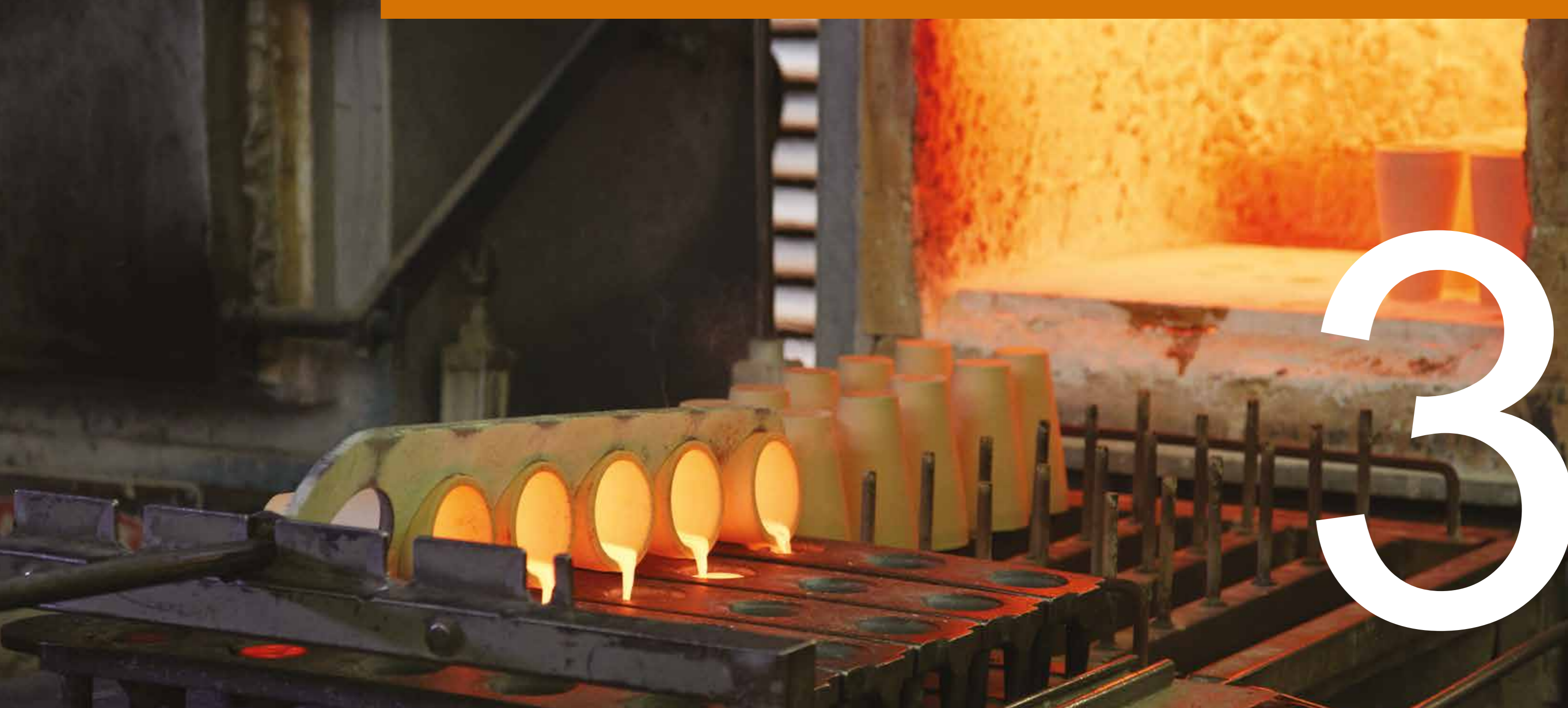
Fire assaying of gold samples at Granny Smith in Australia
